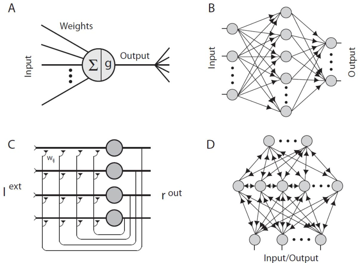
Figure 3: (A) In each node in a neural network, output is a function of the sum of weighted inputs. (B, C, D) Feedforward, recurrent and bidirectional architectures respectively.
